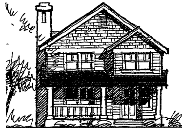
Acceptable condition. Porch roof extended from main roofline
