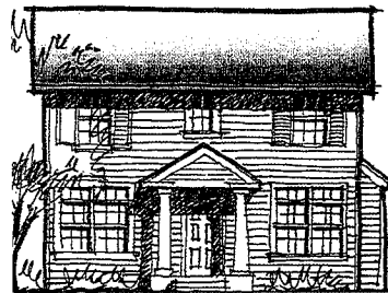
Acceptable condition. Stoop entry covered by transverse gable to break scale of roof down.
