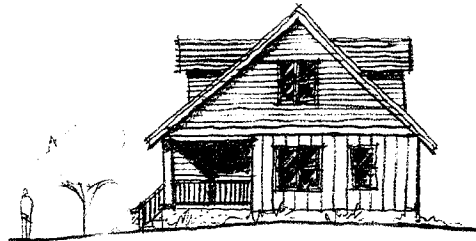
Acceptable condition. Porch area fully covered by main roofline
